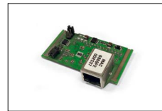
Modulo Ethernet web IB-Lite (COMAP) IB-Lite web Ethernet module (COMAP) Module Ethernet web IB-Lite (COMAP) Modulo Ethernet web IB-Lite (COMAP)
